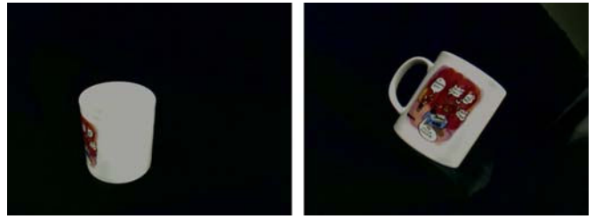
Fig. 5. Snapshots from the experiment. The robot starts with the initial image on the left. The neural network ESC algorithm provides references in order to maximize the texture density and the snapshot on the right is achieved at the final position.
