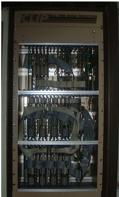
Figure 1: UCL CLIP4 SIMD image processing system
