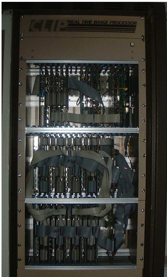
Fig. 1. UCL CLIP4 SIMD image processing system
